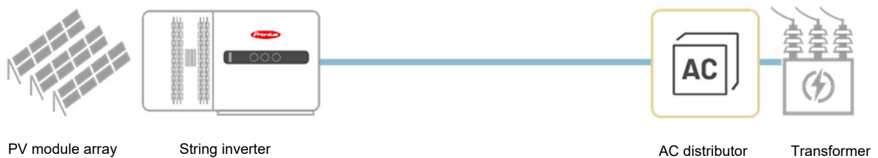
Figure 1: Structure of a decentralised system
